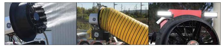
5 Optional Accessories: Misting Ring provides 30 GPM at 60 psi, while optional ducting and LED lights add even more versatility
